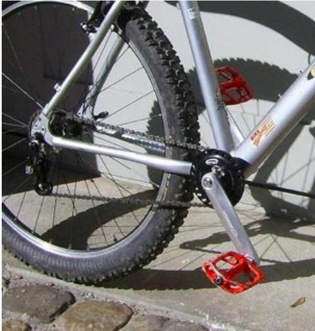
Even less problems with a transversal chainline: high-speed-drive chainring is very small, and therefore short tangential travel, where the chain "enters" the chainring.
