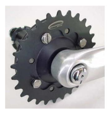
For extrem low gears there is a 27 t. chaining available. It equals a chaining of just 11 t. in low gear mode! It is mounted at the position of the spider.
