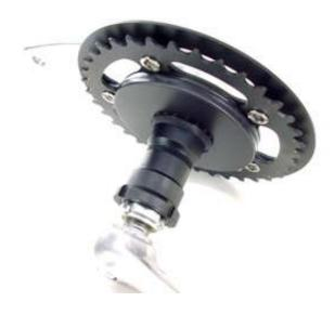
For extrem narrow b.b. shells of 50 mm width (for example on fully faired cabin bikes) we deliver such a version.
