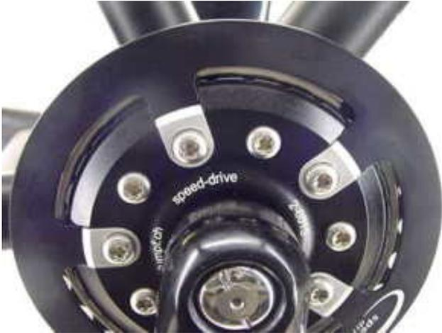
Model "08" has a total of 10 Torx screws on the outer side (for T25 key).
