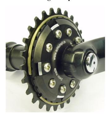
They are hold by a circlip and can be exchanged easily.
