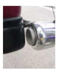
It's so easy: push with the heel of your shoe either on the right or on the left side of the axle on the push button to change from high to low gear or vice versa! That's all!
