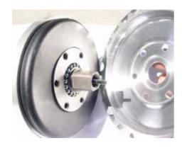
The design allows to strip down the system without any special tools, if ever required.
