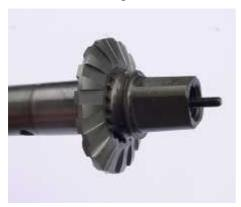
The heart of the *high-speed-drive* gearing system is the "Cargo" clutch, which is switched by pushing the gear shift button either on the left or on the right side.
