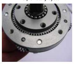
In the centre there is the so called sunwheel. Like planets around the sun, the four planet pinions orbit the sunwheel.
