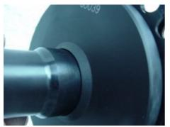
The conical parts of either gear housing and the lock nut center the unit perfectly.
