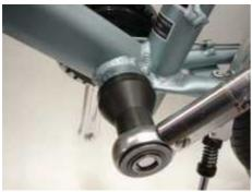
This box spanner can be combined with a 1/2" torque wrench.
