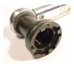
To tighten the lockring, please use the box spanner of our "profi" tool set. It's the easiest way to tighten it with the recommended torque of 100-110 lb ft, which is required to hold the gear housing against the reaction torque. The spanner is guided by the spindle, and provides a safe tightening without the danger of slipping.
