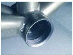
The outer diameter of the conical part must be between 39.0 - 40.0mm.
