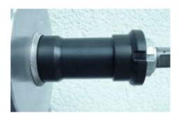
**High-speed-drive** is available with cone rings to fit bottom bracket shells of 33.6 up to 34.5mm of inner diameter.
