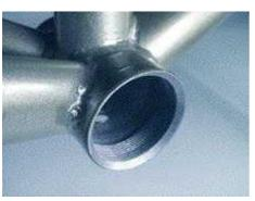
If you want to fit the *mountain-drive* unit without the anti-twisting bracket (torque lever), you must prepare the bottom bracket tube as shown on the left.
