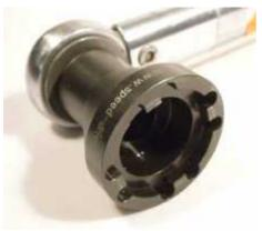
This box spanner can be combined with a 1/2" torque wrench.
