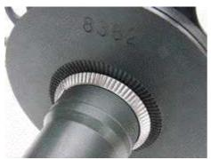
Use aluminum cones for steel bottom brackets, but a knurled steel cone on the right side for aluminum bottom brackets.
