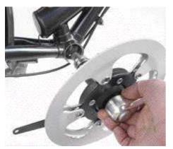
Insert the *mountain-drive* unit in the empty bottom bracket shell. Use shims, which are included in the basic package, to make up for small difference in diameter.
