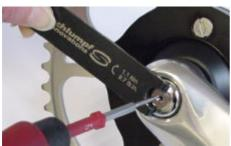
... finally tighten the left gear shift button: hold it with the wrench of our tool set and tighten it with 1.1 Nm.
