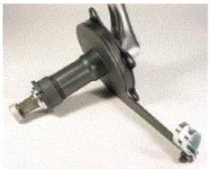
The torque lever is fitted to the rear chainstay with a clamp (included in the shipment).
