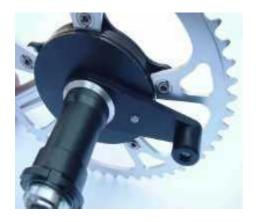
For Brompton folders we offer a special torque lever for *mountain-drive*, which makes the installation even easier.
