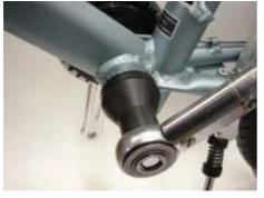
To tighten the lockring, please use the box spanner of tool set "installation and maintenance".
