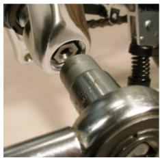
Next step is tightening the left crankarm with a standard 14mm box wrench and a torque of 50-55Nm (40 lbft)...
