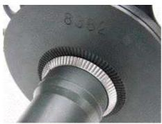
Use an aluminum cone for steel bottom brackets, but a knurled steel cone on the right side for aluminum bottom brackets. Do not install **speed-drive** into thin aluminum bottom bracket shells with wall thickness of less than 3mm. The conical rings exert considerable force that could damage the shell.
