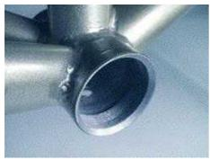
Chamfering the shell to an outer diameter of 39.5 - 40mm
