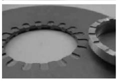
The black plate of the gear housing has milled grooves for the "teeth" of the cone ring. This makes sure, that the cone ring can't spin under heavy load.
