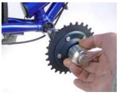
Slide the **speed-drive** into the empty bottom bracket shell and tighten it with a nut on the left side. That's all!
