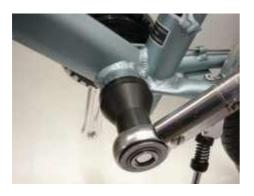
To tighten the lockring, please use the box spanner of tool set 2.
