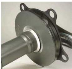
Speed-drive is centered by a conical ring on the right side. On the left side, the nut has a 45° shape to center the unit perfectly within the bottom bracket. **speed-drive** never uses a torque lever. The bottom bracket shell therefore has to be chamfered before the installation.
