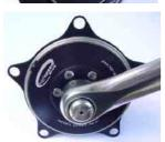
Adapter for BCD130mm. The adapter is fitted to the gear housing like the chainrings above.
