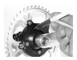
At the assembly, we lube the *mountain-drive* with a basic quantity of MoS2-grease, which is good for at least 2'000 - 3'000 miles.
