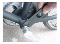
After several thousand miles, please check for bearing play. The chainring must not have any play along the spindle axis. If there is any play, slightly tighten the self-locking nut on the left end of the axle. Never tighten the nut too firmly. Some play between the cranks and chainring in the direction of crank rotation is normal an necessary for proper engagement of the gears after switching.
