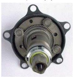
In the centre there is the so called sunwheel. Like planets around the sun, the four planet pinions orbit the sunwheel.
